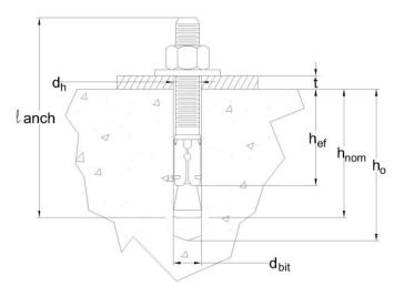
FIGURE 2—US ANCHOR ULTRAWEDGE ANCHOR INSTALLATION
