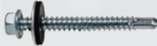
Non-Slotted Hex Washer Head w/Bonded EPDM Washer Self-Drill Screw, Zinc Plated CR+3
