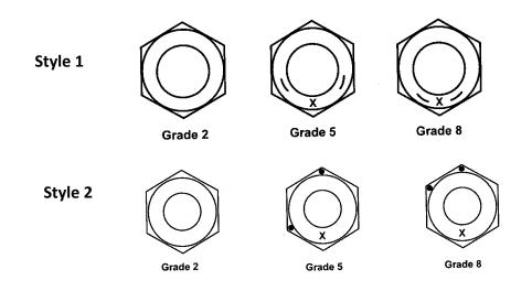
Notes: The nuts will also have manufacturer's marking, in addition to the grade marking as shown above.
