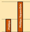
Phillips Square-Driv with ACR offers more than twice the driving torque than a standard Phillips screw driven with the same end load. #8 screw (1lb end load) = 41 inch pounds
